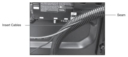
Figure 11: Inserting Cables into the Wire Loom
