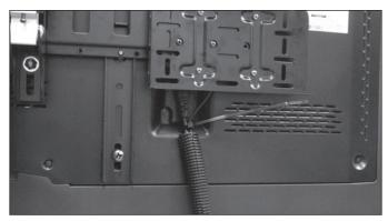
Figure 14: Inserting PC Power Cord and Display Monitor Cord (example only)
