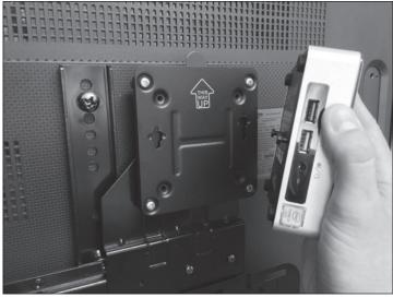
Figure 6: Attaching Screws to Back of the Computer (Left)
