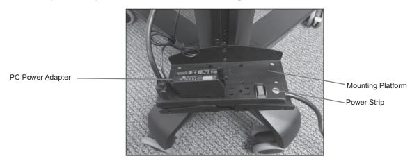
Figure 10: Mounted PC Power Adapter and Power Strip
